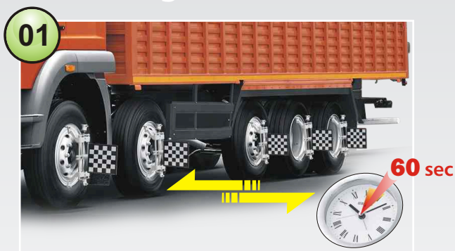
One shot Runout Compensation
